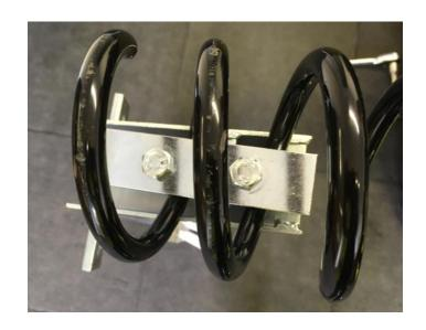
3. Repeat steps 1 and 2 to fix the horizontal brush onto the other end of the spring.
